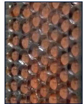
Complete Penetration of Magnet Wire
